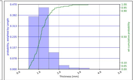
Fig. 6: Distribution density (q1) of the width, weighted by length
