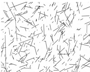
Fig. 1: Single rCF scanned at 3200 dpi
