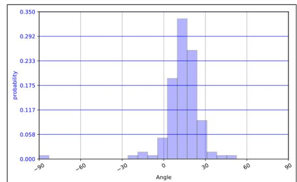
Fig. 9: Orientation - Distribution density (q1) of the angles of the wrappers
