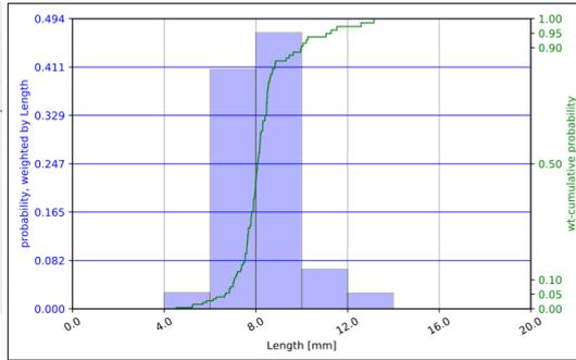
Fig. 5: Distribution density (q1) of the length of roving snippets, weighted by length
